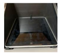
Place the third L bracket at the top of the device, on the hood- at or near the center without blocking the camera hole if there is one.
