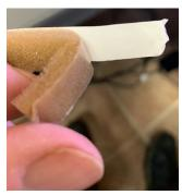
4. Press the tape onto the hood to block the light.
