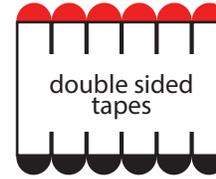
Use the enclosed double-sided tape to hold the filter in place. As screens vary in size and shape, use your best judgement as to the best placement of the tapes. Use the guidelines below.
