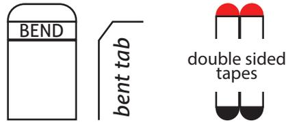
**5. Bend Tabs:** Bend tabs at scored seams. Remove backing to expose adhesive and press firmly to frame of monitor in six places (see illustration A). Place upper tabs a few inches from the top corners (as shown). This allows the filter to be easily pulled out from the top if needed. Do not place bend tabs along top edge.
