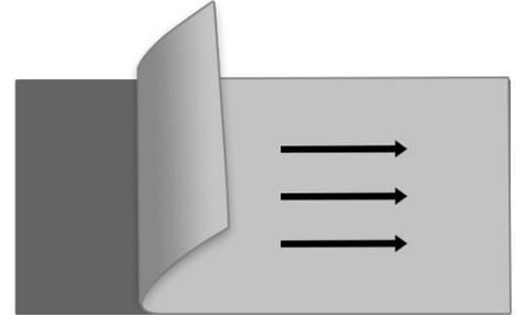
**Note: The Privacy Filter is to be installed matte side out.**
