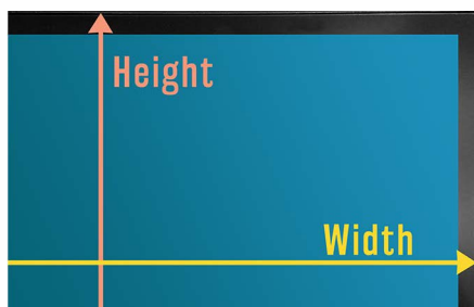
Frameless Device - Measure to the inside edges
